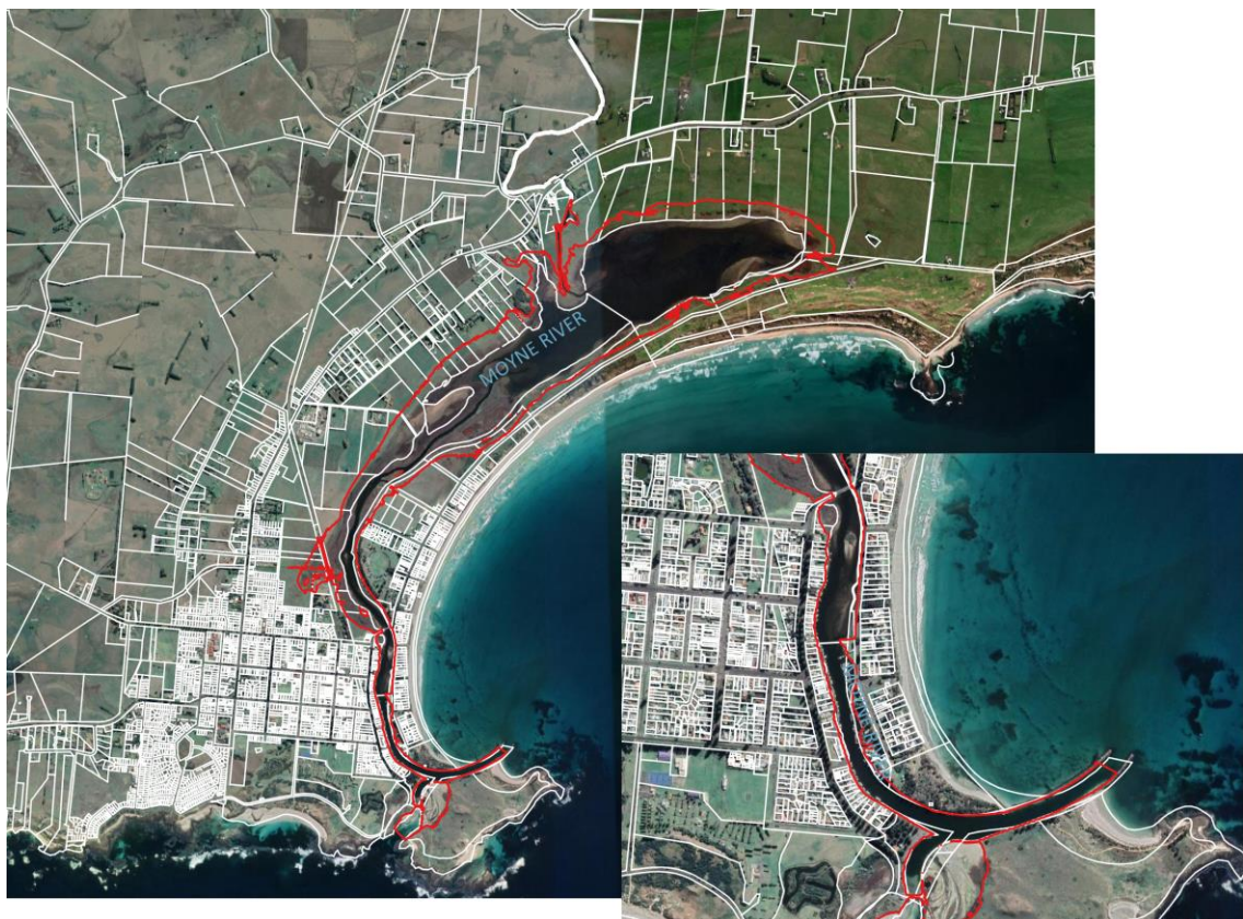
Figure 16 Flood Map for Port Fairy for the 1% AEP storm tide, current mean sea level (bathtub modelling, from Water Technology, 2010)
