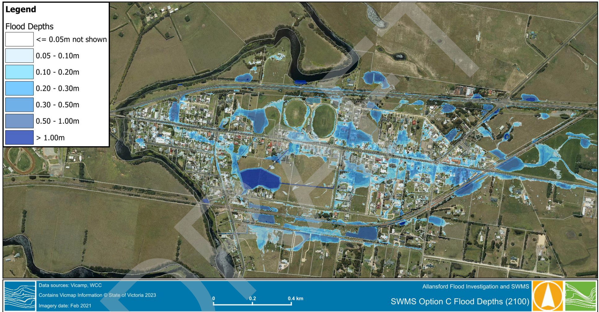
Figure 5-10 SWMS Option C – 1% AEP SSP5-8.5 2100 Flood Depths
