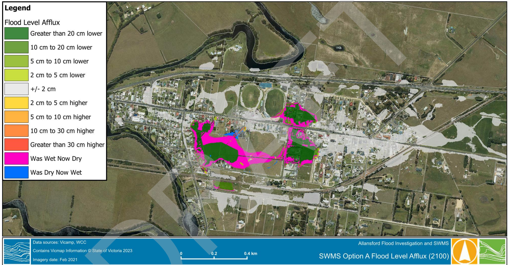
Figure 5-5 SWMS Option A – 1% AEP SSP5-8.5 2100 Flood Level Afflux
