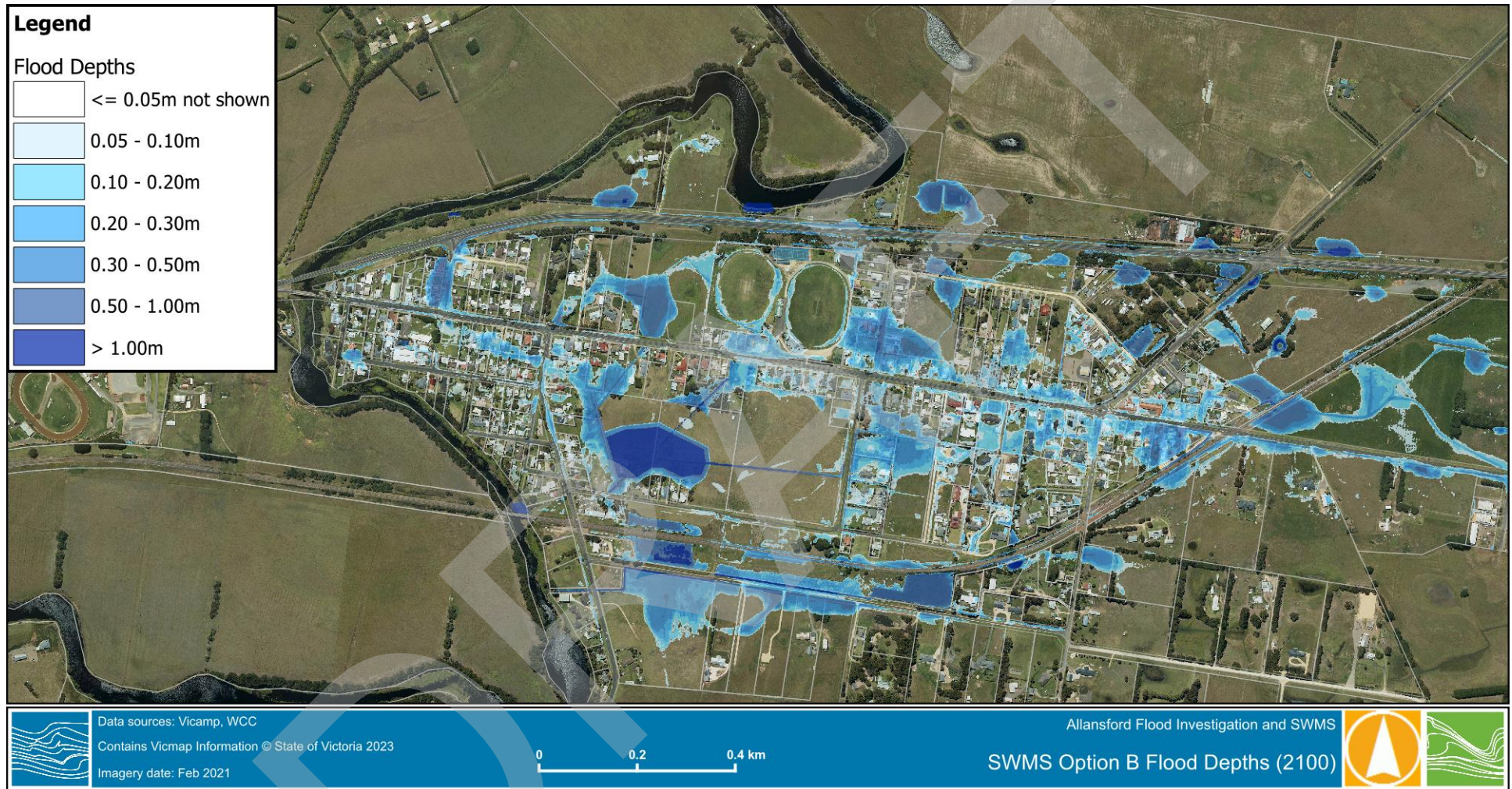
Figure 5-7 SWMS Option B – 1% AEP SSP5-8.5 2100 Flood Depths
