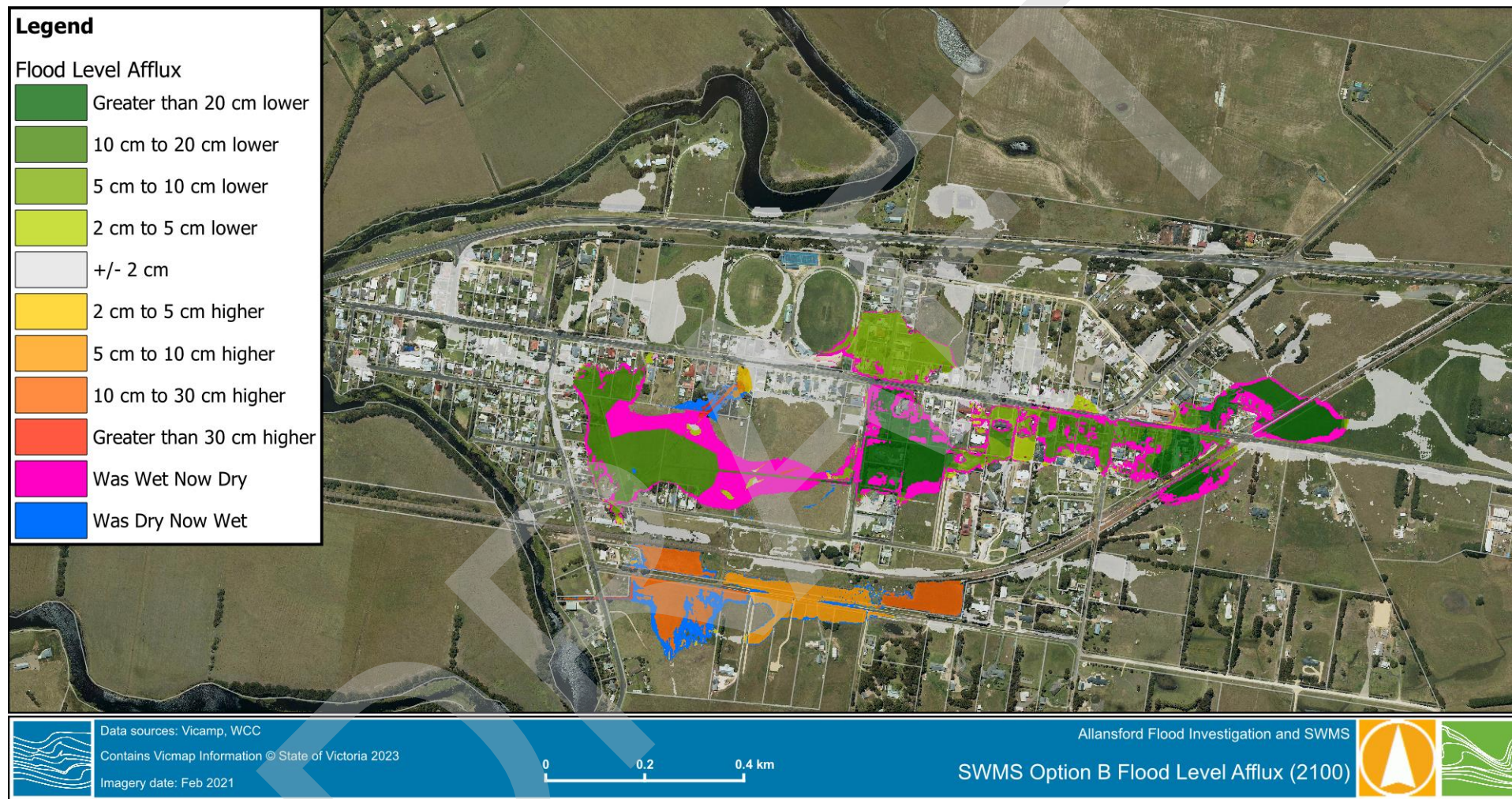
Figure 5-8 SWMS Option B – 1% AEP SSP5-8.5 2100 Flood Level Afflux
